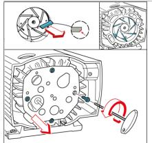
The sliders are also installed behind the front cover. Loosen and remove them as described in the previous point.
