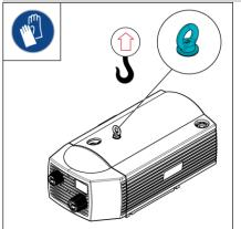
The pump may only be attached to the eyebolt. The following must be observed:
