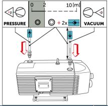
Make the pipes at least as large as the nominal diameter of the connection.
