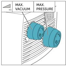
The pump is equipped with a vacuum regulating valve, which allows the vacuum required for the application to be set.
